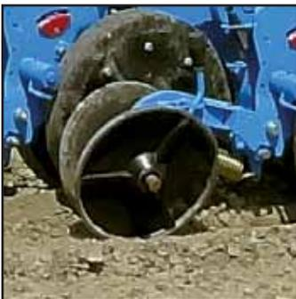
The new cast iron press wheel is 9 lbs per wheel lighter than old cast iron closing wheel. The new wheel has the same diameter size and pitch angle as the previous design.
