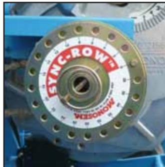
Sync-Row® is a Monosem patented seed stagger timing system for Twin-Row. Sync-Row® provides consistent diamond pattern seed drop for maximum space between plants.
