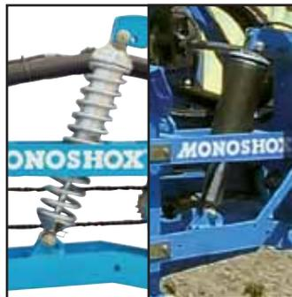
Monoshox® and Monoshox® Air downforce systems are adjustable down pressure with gas filled shock to dampen unit bounce & help maintain consistent planting depth.
